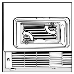
■ Turn both levers on the condenser unit to the vertical position.
